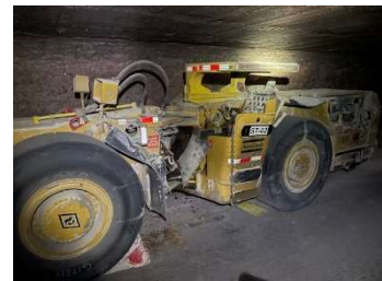
ST-02 Atlas Copco ST3.5 Scoop Tram
